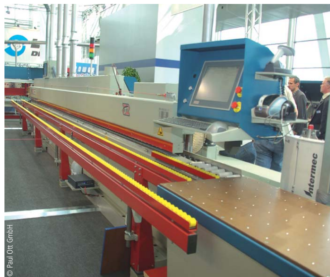
Reliable automation solutions, even for tiny batches, are available from Paul Ott (picture above: the edge-banding machine).
