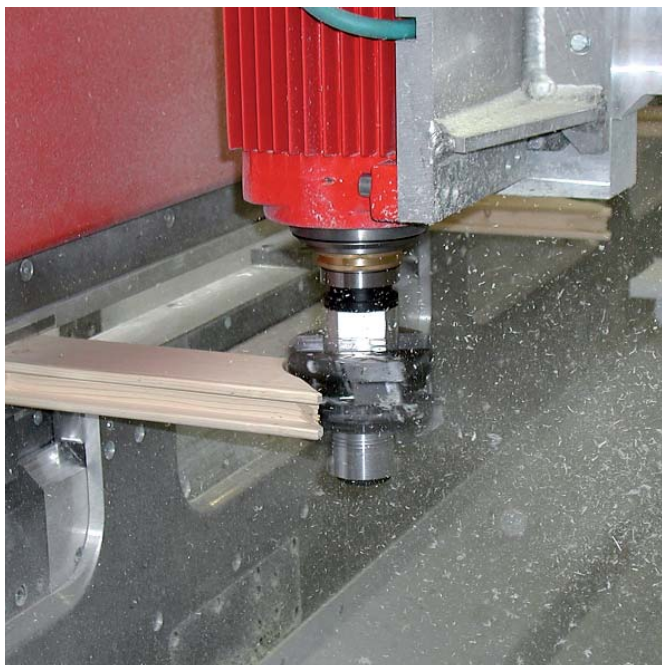
At Fill, a machine-engineering company, CAD data can be entered directly into the finishing system for wood preforms and passed on to the control system via an interface.
