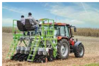
©wintersteiger, Dynamic Disc Plus precision spaced planter
