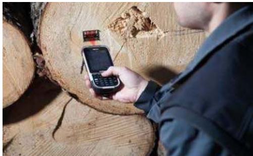
© Latschbacher, Industry line tag and mobile data collection device
