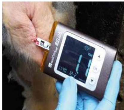
© Schreinecke, WellionVet BELUA meter - Measurement of ketones in the blood of cows
