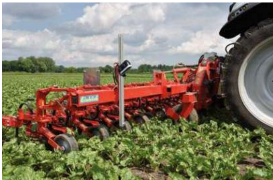
© Einböck GmbH, Row Crop Cultivator with camera steering system CHOPSTAR with ROW GUARD
