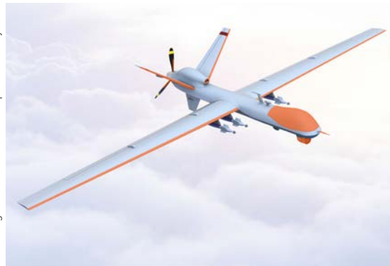
Orange marked areas = ice protection system
