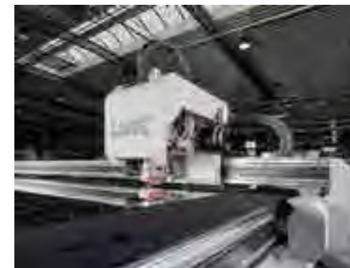
高效的平板玻璃自动切割设备 High performance machine for automatic cutting of flat glass
