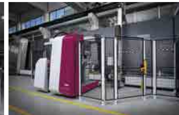
中空玻璃生产线热塑暖边条 (TPA) Insulating glass line for thermoplastic spacers (TPA)
