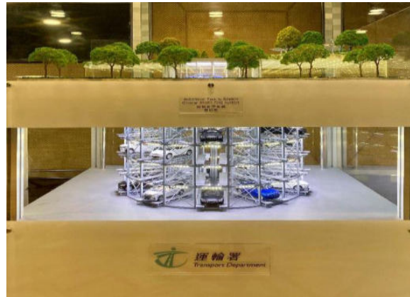
Circular Shaft Lifting System
