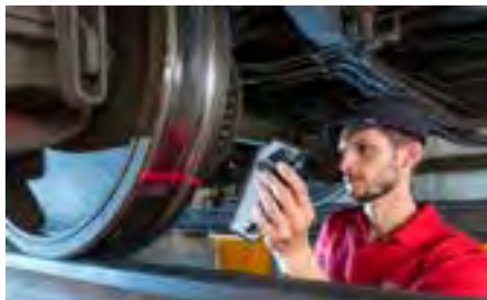
高精度的车轮轮廓测量 high-precision wheel profile measurement
