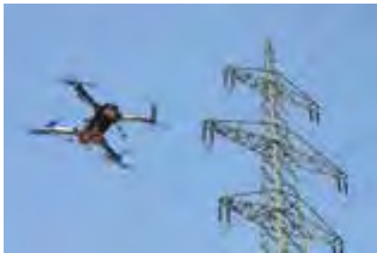
搭载 RICOPTER 的 RIEGL VUX-240 激光雷达，应用于无人机测绘工程 RICOPTER with RIEGL VUX-240 LiDAR Sensor for UAV-based surveying missions
