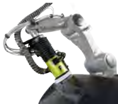
利用活动轨道装备（AOK）进行接触敏感性砂磨和抛光 Contact-sensitive sanding and polishing with Active Orbital Kit (AOK)
