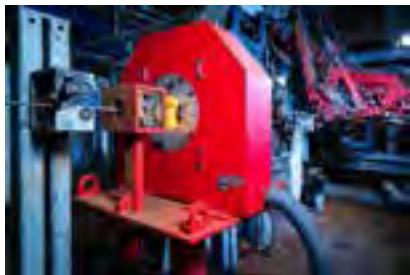
线材、棒材和钢筋的圆形截面的连续内线监测 continuous inline monitoring of round cross-sections for wire, rod and bars
