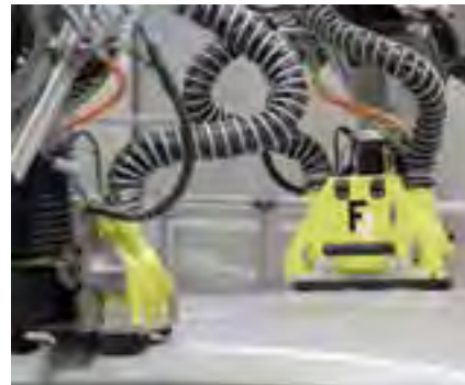
活动式敏感套件（ASK） Active Sensitive Kit (ASK) for roof joint grinding and door entry brushing
