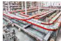
适用于扁平或小包装物品的高效科纳普分裂式托盘分拣系统 Efficient KNAPP Split Tray Sorting System for flat-packed or small items
