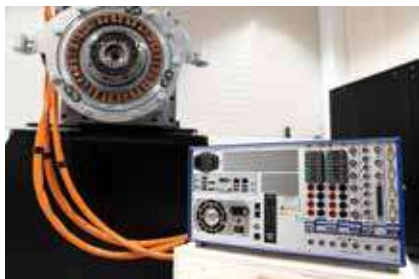
德维创电机动力总成测试台功率分析仪 DEWETRON Power Analyzer for E-Motor Powertrain Testbench
