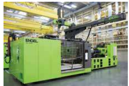
在上海工厂内，ENGEL正在建造大型两板duo系列 机器设备。 In the Shanghai plant, ENGEL is building large-scale machines of the dual platen series duo.
