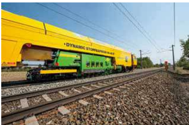
09-4X E 3 动态捣固快车：环保与可持续发展。 09-4X E 3 Dynamic Tamping Express: environmental protection and sustainability.
