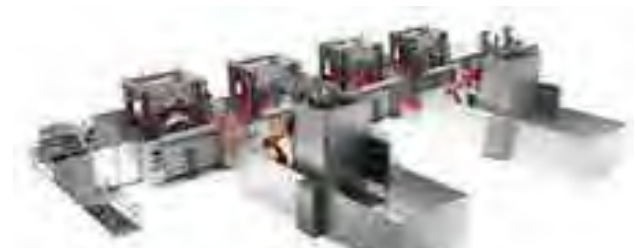
全自动差压铸造生产线 Fully automated counter pressure casting line
