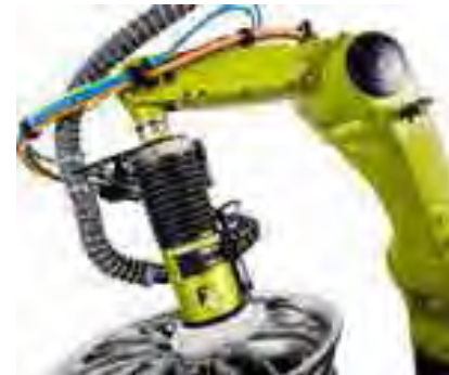
利用活动轨道装备（AOK）进行 接触敏感性砂磨和抛光 Contact-sensitive sanding and polishing with Active Orbital Kit (AOK)
