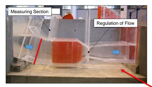
Optimization - Capacity 3%-5% Shape of approach flow channel Transition – Change in inclination Trash Rack
