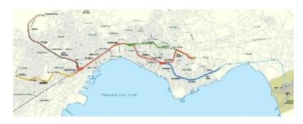
The extension of the subway to Kalamaria (Section Patrikiou - Mikra) has a length of 4.5 km and consists of two single-track tunnels TBM with 5 stations. It is the first section of a track that is to be guided to the international airport.
