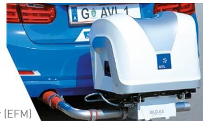
AVL M.O.V.E. Exhaust Flow Meter (EFM)
