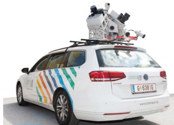
© JOANNEUM RESEARCH, Mobile mapping system, mounted on the car
