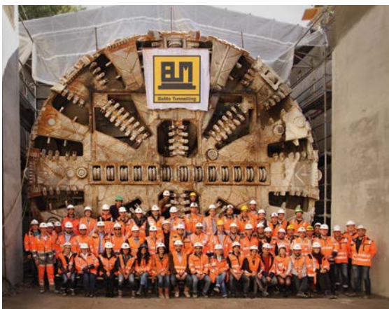
Slurry TBM with BeMo team, Metro Karlsruhe, Germany
