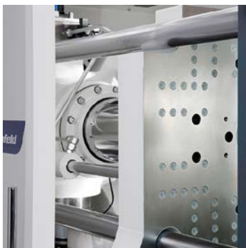
Lubrication-free tie-bar system © Wittmann Battenfeld
