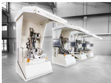
Manual measurement and straightening plant © Klaus Mitterhauser Fotografie
