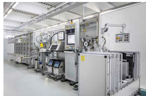
Fibre ribbon production line FRP 05 © 2018 Paul Sebesta
