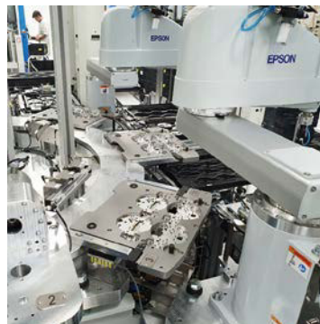
Automatic test platform for electronic assemblies
