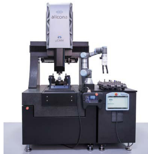
Optical CMM machine as a Pick & Place system all pictures © Bruker Alicona
