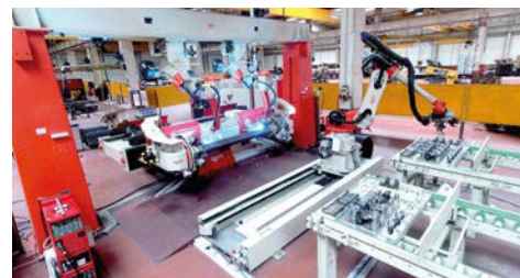
Cooperating robots in welding cell for truck axles
