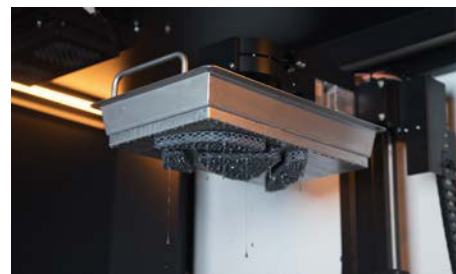
Construction platform with print part
