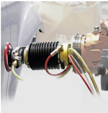
Automated contact-sensitive grinding of car body
