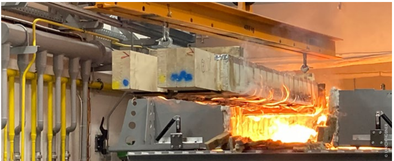
BRANDPRÜFUNG IM RAHMEN VON MECHANICAL PROPERTIES OF WOOD FOR FIRE DESIGN AN DER ETH ZÜRICH • FIRE TESTING AS PART OF THE 'MECHANICAL PROPERTIES OF WOOD FOR FIRE DESIGN' AT ETH ZÜRICH
