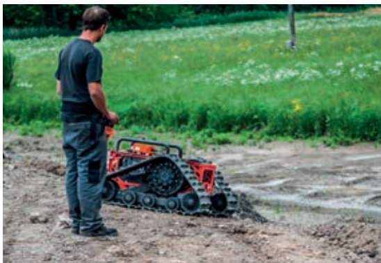
Robotic platform BOCK: Electric transport, power
