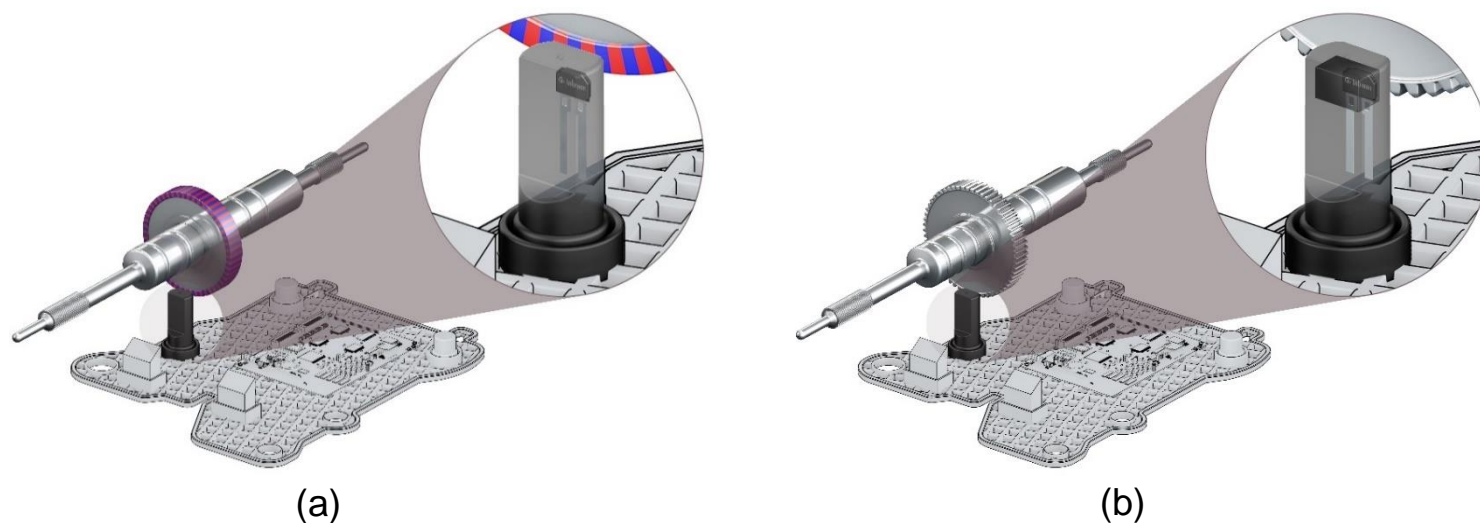
Typical sensing arrangement for wheel speed measurement (a) pole wheel with sensor (b) toothed wheel with sensor and back-bias magnet
