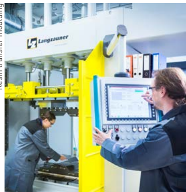
Resin transfer moulding
