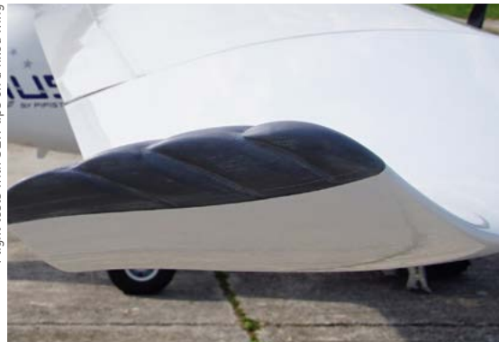
Flight tests with SEW tips on a fixed wing
