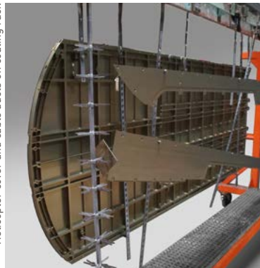
Helicopter cover and cable ducts on coating rack
