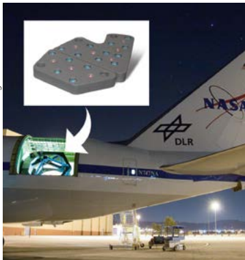
Black coated titanium fittings for mirror cells
