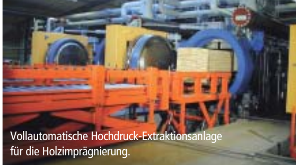
Full automatic high-pressure extraction plant for the wood injection.
