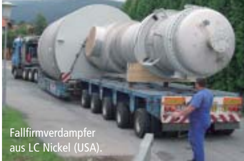
Falling film evaporator from LC-nickel (USA).
