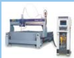
2D WJC plant by aps with integrated high-pressure pump.
