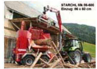
Wood shredder for biomass utilization
