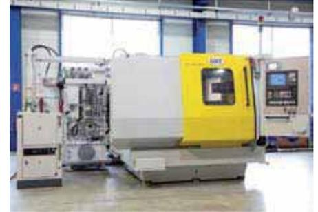
Workpiece-specific cylindrical grinding machines
